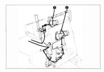
In case of three threads, pass under looper thread 1 first, over looper thread 2 second, and finally needle thread 3 as shown at right.
